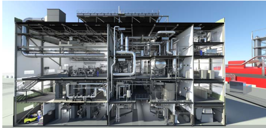
Figure – 3D model of 32 MW th (90 bar(g) 500 °C) CHP for Härjeåns Energi in the very north of Sweden. This plan can also be operated in condensing mode for maximizing of power output.
